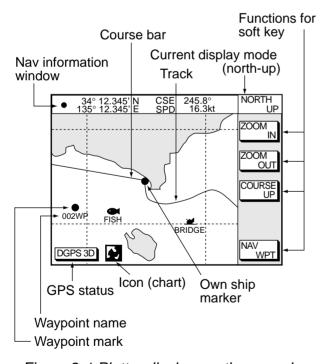
Figure 2-1 Plotter display, north-up mode
